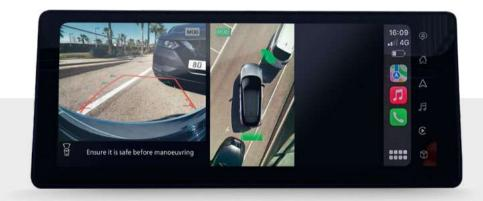
From the single-camera Rear View Monitor to the virtual birds eye view 360° composite view of the Intelligent Around View Monitor, Nissan Intelligent Mobility gives you the confidence to manoeuvre and park like a pro every time. help make these tasks quick and easy. Moving Object Detection alerts the driver with audio and visual warnings if movement around your vehicle is detected.
